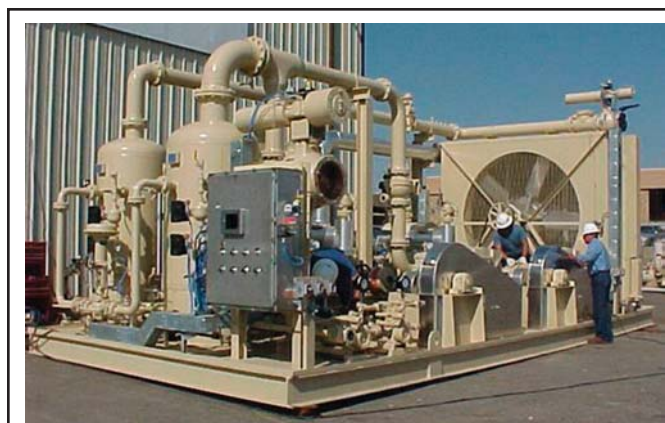
Vapor recovery units are designed to capture high-Btu content vapors that would otherwise be vented to the atmosphere, and turn them into a valuable revenue stream while simultaneously minimizing regulatory and liability exposures.
