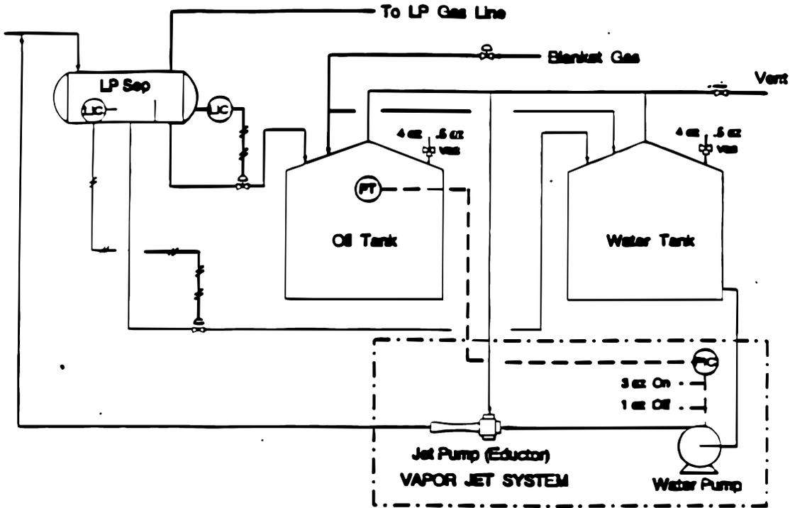
Figure 1 Schematic – Vapor Jet Vapor Recovery System
