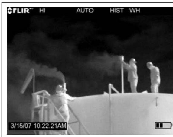
In addition to imaging vent gas from oil storage tanks, compressors and other production equipment, the infrared camera can help prevent safety hazards from exposure to hydrogen sulfide and ignition sources. In this example, workers replacing a leaking valve on top of an oil storage tank were unaware that gas was exiting the tank through the 3.0-inch pipe until the camera captured this image. The latest field video from Hy-Bon Engineering is available at [www.hy-bon.com](http://www.hy-bon.com).
