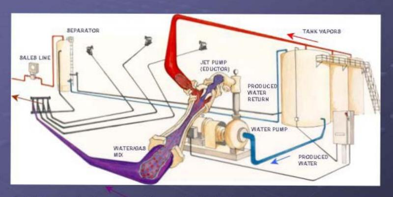
In this patented process, the venturi jet of water pulls tank vapors into the water stream. The gas/water mixture is returned to the separator, where the gas stream breaks out of the water and is produced down the sales line. The water is recirculated back to the tanks in a closed loop system.
