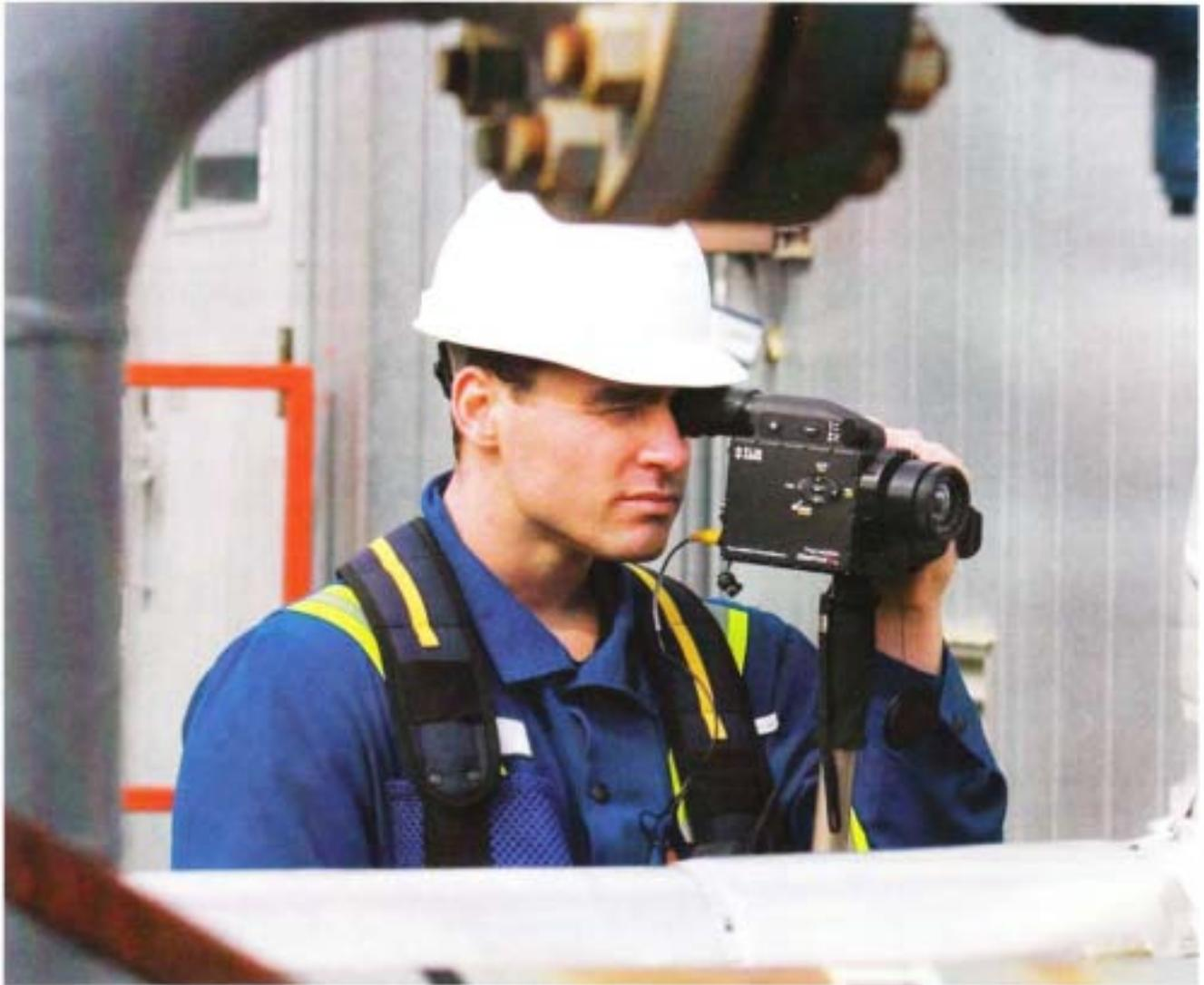
Engineer Terence Trefiak of Target Emissions Services scans for fugitive emissions with a FLIR GasFindIR thermal imaging video camera. The infrared camera delivers real-time thermal images of gas leaks. *Mike Ridevaad photo.*
