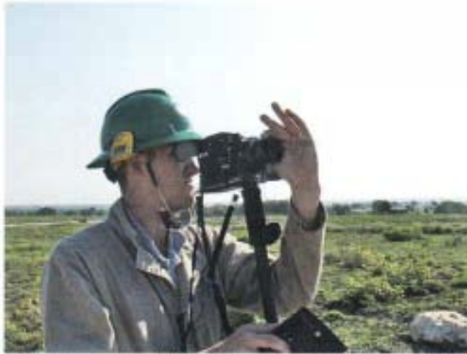
A technician uses the FLIR GasFinder camera to identify gas emissions. Hy-Bon Engineering photos.
